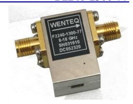
F2240-1300-77 is a single junction coaxial isolator with SMA female coaxial connectors operating in the frequency range from 8.0GHz to 18.0GHz and offers 0.8dB typical insertion loss and 16dB typical reverse isolation. The coaxial isolator can handle 10 watts of forward CW power and 1 watts of reverse power.
